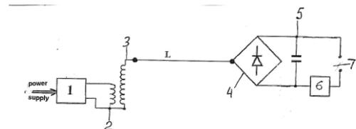
**Fig. 13. The scheme of the resonant high-frequency mono-wire electric transmission system (Krasnyansky's project [31])**
