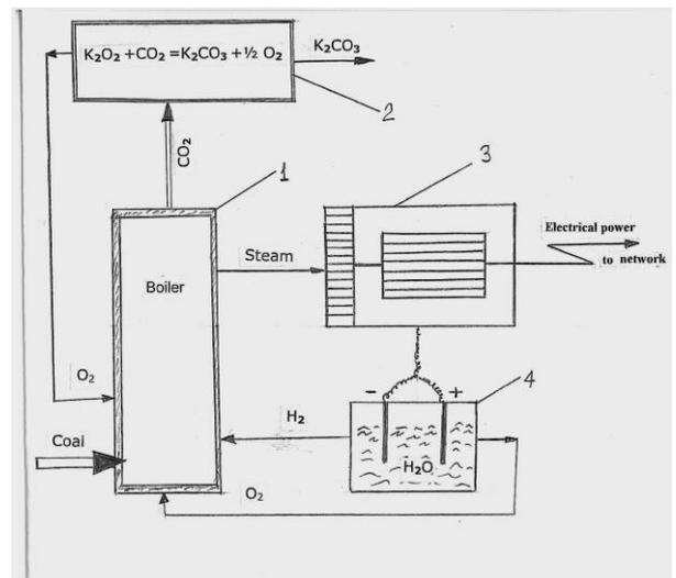
**Fig. 5. Scheme of the coal clean incineration**
