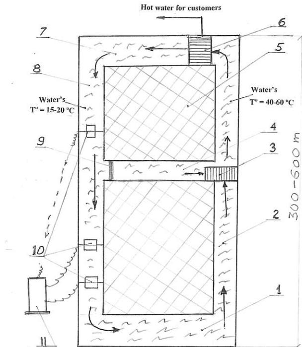
**Fig. 7. Scheme of recycling of thermal and kinetic energy for the mine's waters**
