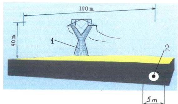
**Fig. 12. Comparison of an usual high-voltage line (1) and the superconductor electricity pipeline (2)**
