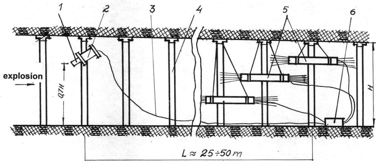
**Fig. 10 - Automatic system for the suppression of explosions using PSE-powder:**
