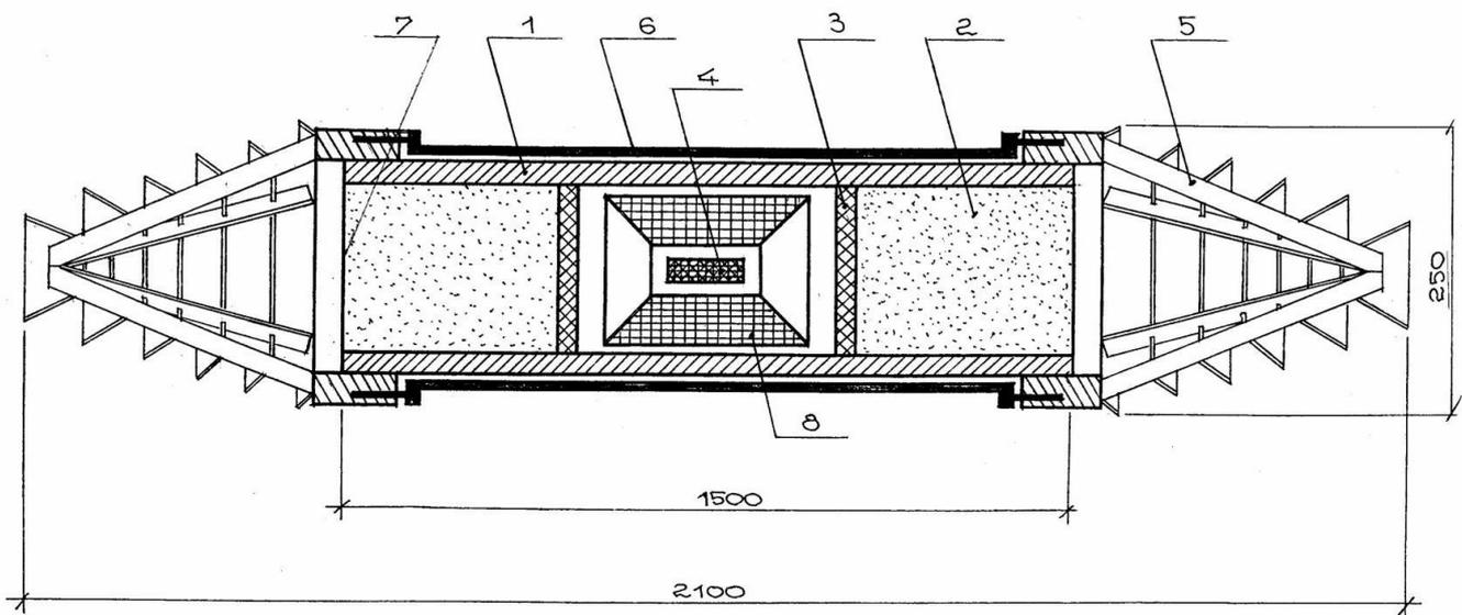
**Fig. 8. - Automatic double-action explosion suppressor:**
