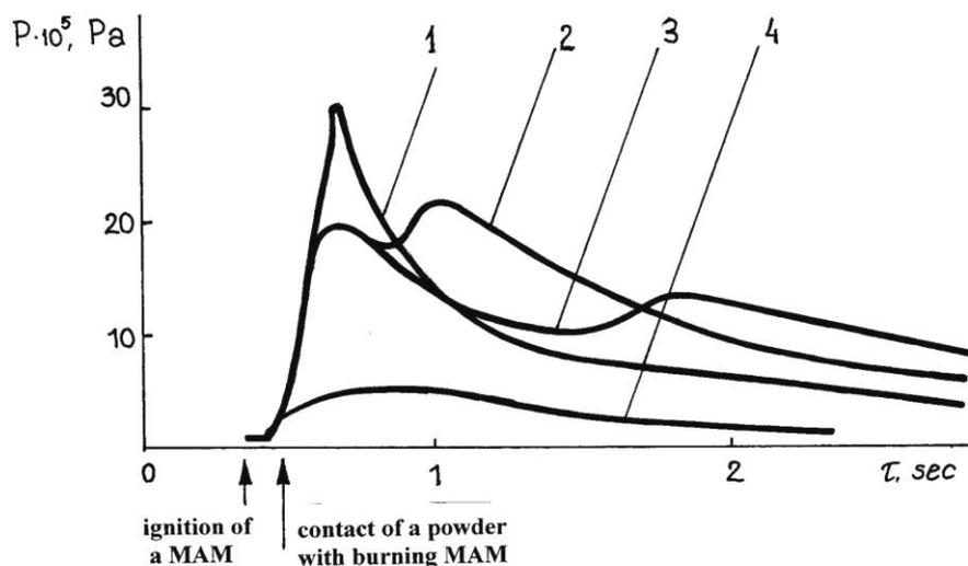
**Fig. 5 - Suppression of the developed methane-air mixture explosion (MAM) by "PSE"-powder in a laboratory tube:**
